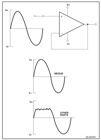
Figure 5. In a Non-Inverting Voltage-Follower Configuration, the NE5230 will Give Full Rail-to-Rail Swing. Other Low Voltage Amplifiers will not Because they are Limited by their Input Common-Mode Range and Output Swing Capability.
