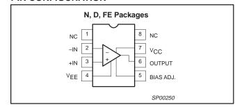
Figure 1. Pin Configuration
