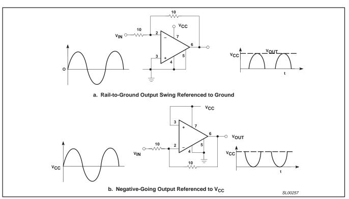
Figure 8. Half-Wave Rectifier With Positive-Going Output Swings
