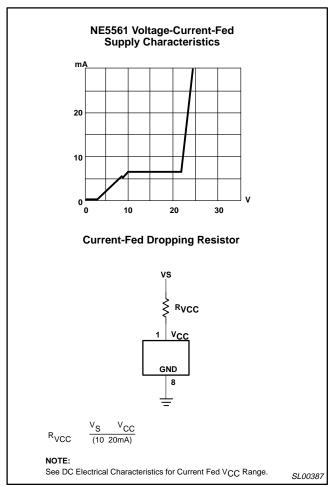
Figure 4. NE5561 Voltage-Current-Fed Supply Characteristics
