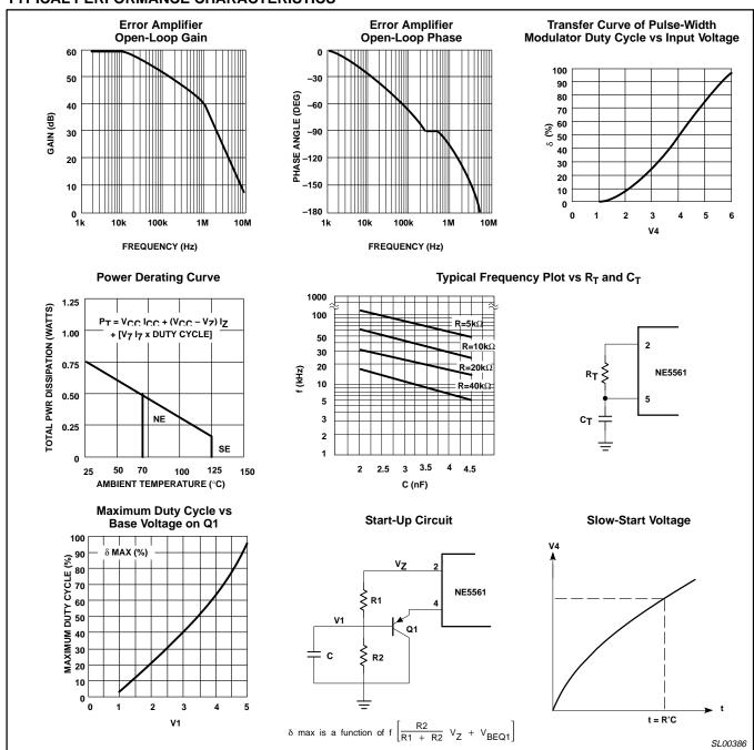
Figure 3. Typical Performance Characteristics
