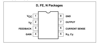
Figure 1. Pin Configuration
