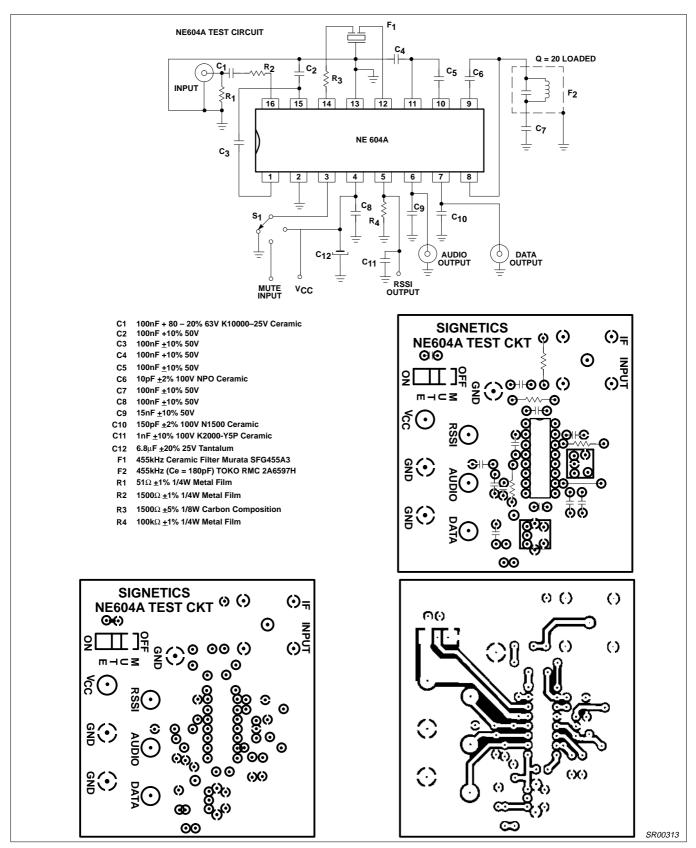
Figure 3. NE/SA604A Test Circuit
