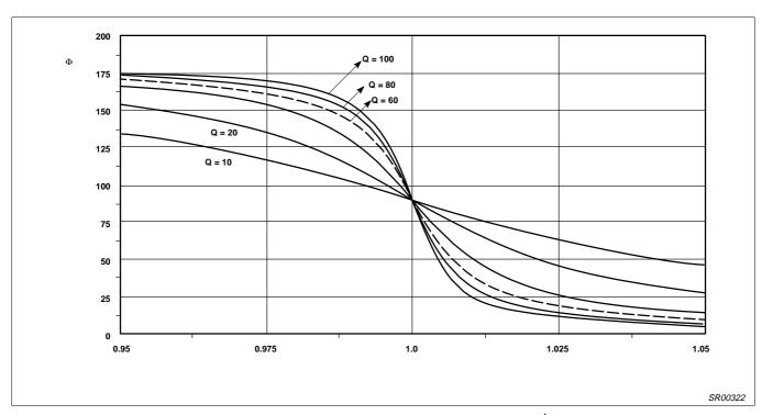
Figure 12. Phase vs Normalized IF Frequency  $\frac{\omega}{\omega_1} = 1 + \frac{\Delta \omega}{\omega_1}$
