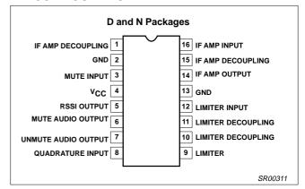
Figure 1. Pin Configuration
