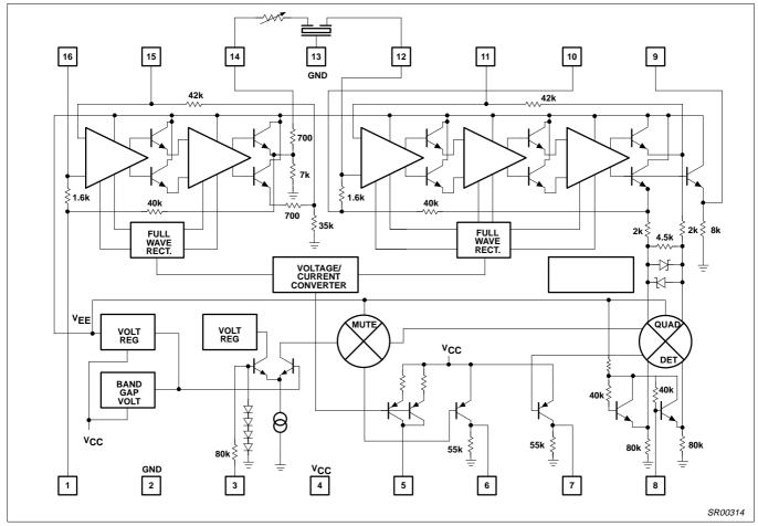
Figure 4. Equivalent Circuit
