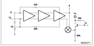
Figure 7. Second Limiter and Quadrature Detector
