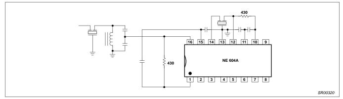
Figure 10. Crystal Input Filter with Ceramic Interstage Filter
