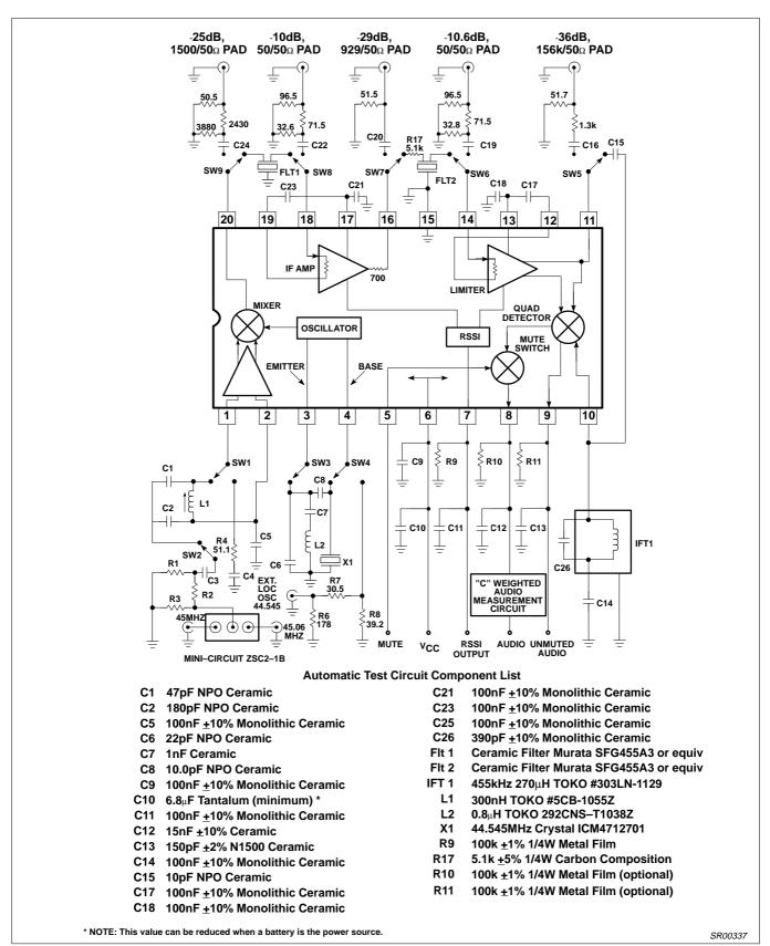
Figure 3. NE/SA605 45MHz Test Circuit (Relays as shown)
