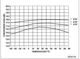
Figure 11. Conversion Gain vs Supply Voltage
