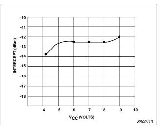
Figure 15. Input Third-Order Intermod Point vs V<sub>CC</sub>
