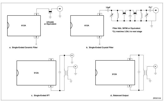
Figure 6. Output Configuration
