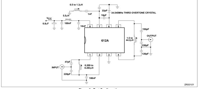
Figure 3. Test Configuration
