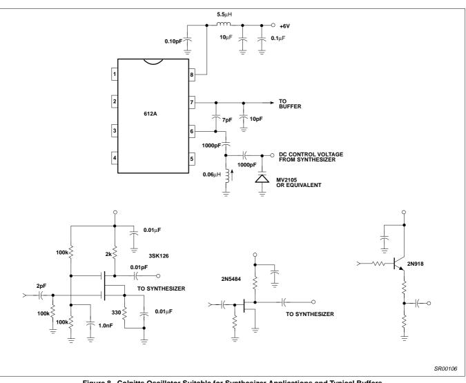
Figure 8. Colpitts Oscillator Suitable for Synthesizer Applications and Typical Buffers
