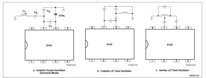
Figure 7. Oscillator Circuits
