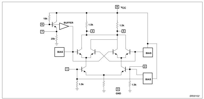
Figure 4. Equivalent Circuit
