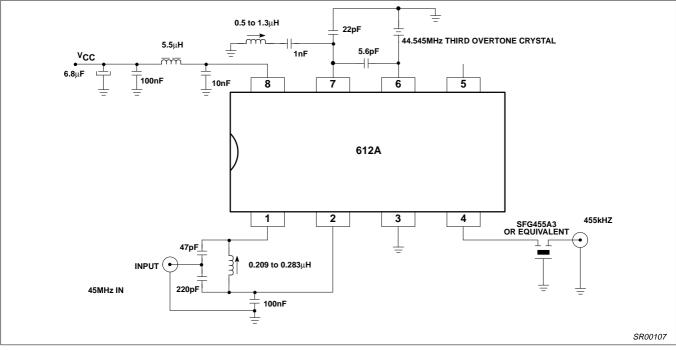
Figure 9. Typical Application for Cordless/Cellular Radio
