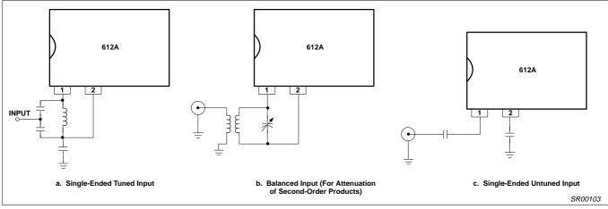
Figure 5. Input Configuration
