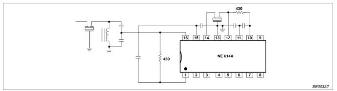
Figure 10. Crystal Input Filter with Ceramic Interstage Filter
