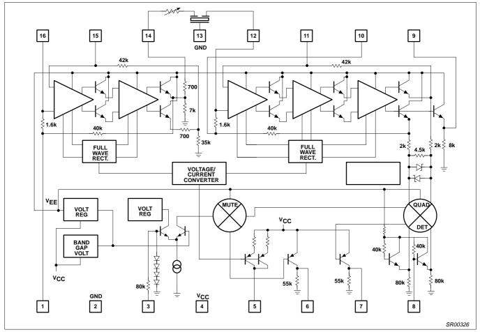
Figure 4. Equivalent Circuit
