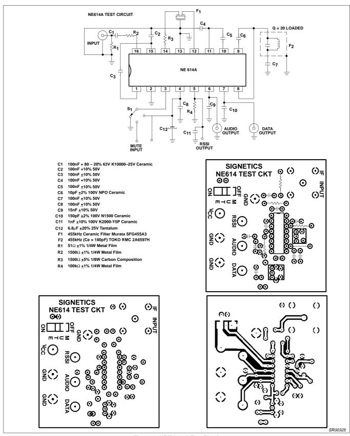
Figure 3. NE/SA614A Test Circuit
