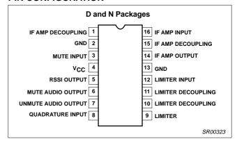
Figure 1. Pin Configuration
