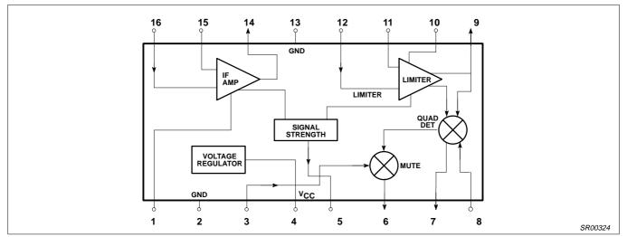
Figure 2. Block Diagram
