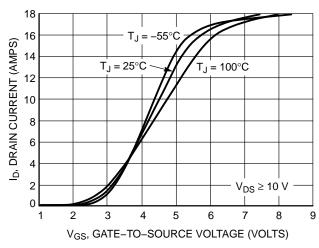
Figure 2. Transfer Characteristics
