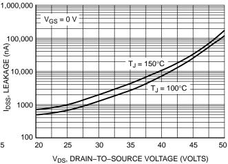
Figure 6. Drain-to-Source Leakage Current versus Voltage
