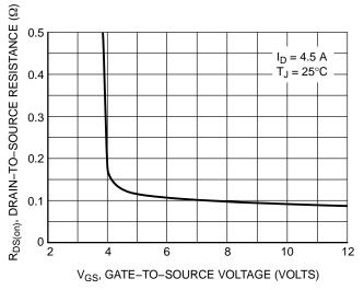
Figure 3. On–Resistance versus Gate–to–Source Voltage
