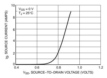
Figure 10. Diode Forward Voltage versus Current
