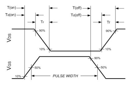
Figure 1. Switching Characteristics Waveforms and Symbols
