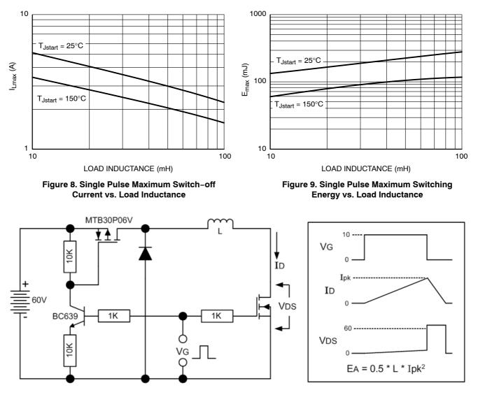
Figure 10. Single Pulse Peak Drain Current and Avalanche Energy Test Circuit
