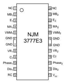
Figure 2. Pin configuration
