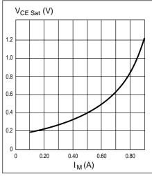
Figure 12. Typical lower transistor saturation voltage vs. output current
