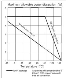
Figure 11. Maximum allowable power dissipation
