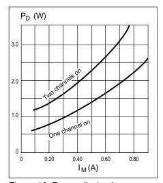
Figure 10. Power dissipation vs. motor current. $T_a = 25$ °C
