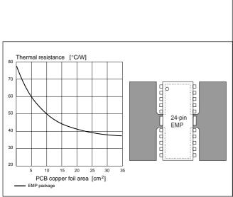
Figure 8. Typical thermal resistance vs. PC Board copper area and suggested layout
