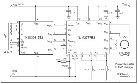
Figure 7. Typical microstepping application with NJU39612
