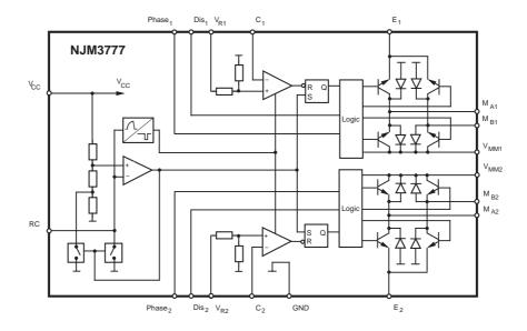
Figure 1. Block diagram
