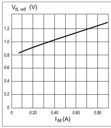
Figure 15. Typical upper diode voltage drop vs. recirculating current
