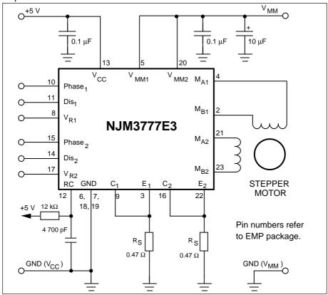
Figure 6. Typical stepper motor driver application with NJM3777
