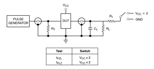
Figure 4. Test Circuit
