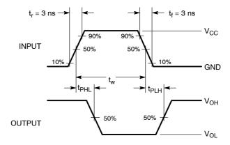
Figure 3. AC Waveforms
