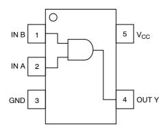
Figure 1. Pinout (Top View)
