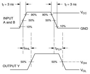
Figure 3. Switching Waveform
