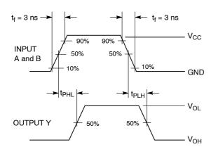
Figure 4. Switching Waveform
