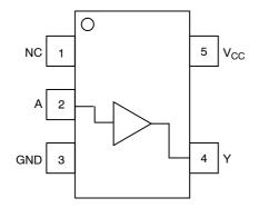
Figure 1. Pinout (Top View)
