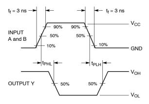
Figure 3. Switching Waveform
