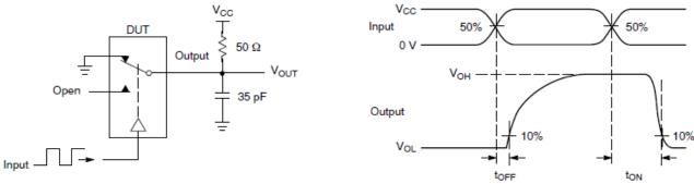
Figure 7. t<sub>ON</sub> / t<sub>OFF</sub>
