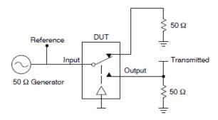
Channel switch control/s test socket is normalized. Off isolation is measured across an off channel. On loss is the bandwidth of an On switch.  $V_{\rm ISO}$ , Bandwidth and  $V_{\rm ONL}$  are independent of the input signal direction.
