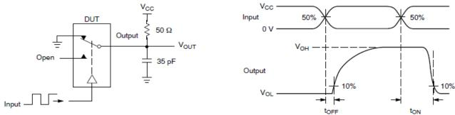
Figure 8.  $t_{ON}$  /  $t_{OFF}$
