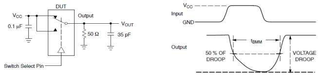
Figure 6. t<sub>BBM</sub> (Time Break-Before-Make)
