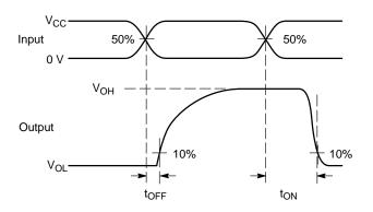
Figure 5. t<sub>ON</sub>/t<sub>OFF</sub>
