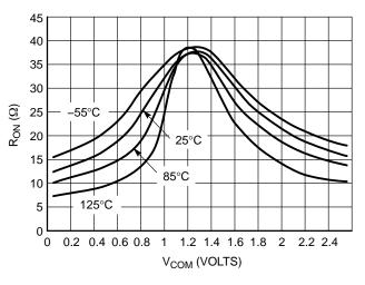
Figure 10.  $R_{ON}$  vs.  $V_{COM}$  and Temperature,  $V_{CC}$  = 2.5 V
