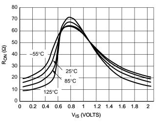
Figure 9.  $R_{\mbox{\scriptsize ON}}$  vs.  $V_{\mbox{\scriptsize COM}}$  and Temperature,  $V_{\mbox{\scriptsize CC}} = 2.0~\mbox{\scriptsize V}$
