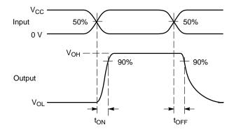
Figure 4. t<sub>ON</sub>/t<sub>OFF</sub>
