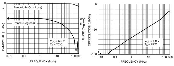
Figure 14. ON Channel Bandwidth and Phase Shift Over Frequency
