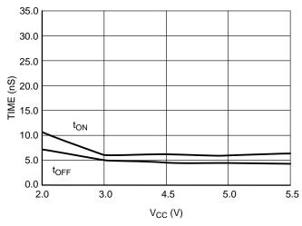
Figure 13. Switching Time vs. Supply Voltage, T = 25°C
