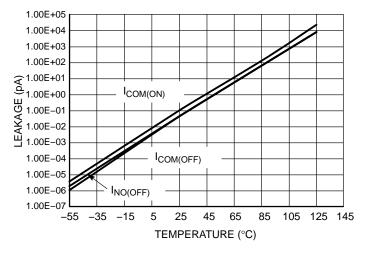
Figure 3. Switch Leakage vs. Temperature
