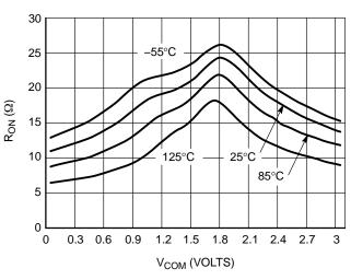
Figure 11. R<sub>ON</sub> vs. V<sub>COM</sub> and Temperature,  $V_{CC}$  = 3.0 V
