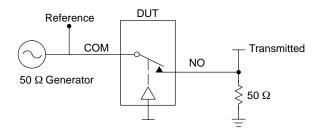
Channel switch control/s test socket is normalized. Off isolation is measured across an off channel. On loss is the bandwidth of an On switch.  $V_{\rm ISO}$ , Bandwidth and  $V_{\rm ONL}$  are independent of the input signal direction.
