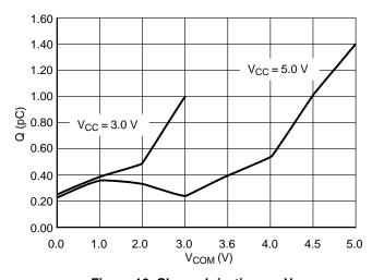
Figure 16. Charge Injection vs.  $V_{COM}$
