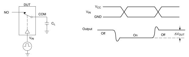
Figure 7. Charge Injection: (Q)
