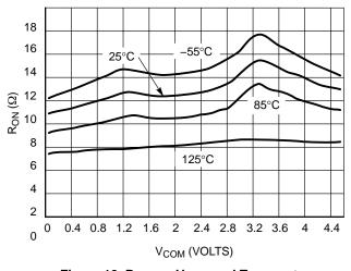
Figure 12.  $R_{ON}$  vs.  $V_{COM}$  and Temperature,  $V_{CC}$  = 4.5 V
