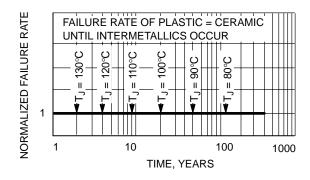
Figure 2. Failure Rate vs. Time Junction Temperature
