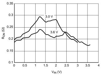
Figure 12. On-Resistance vs. Input Voltage
