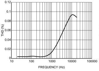
**Figure 9. Total Harmonic Distortion**
