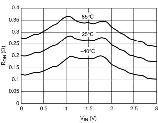
Figure 10. On–Resistance vs. Input Voltage  $@V_{CC} = 3.0 \text{ V}$
