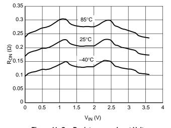
Figure 11. On–Resistance vs. Input Voltage @ V<sub>CC</sub> = 3.6 V
