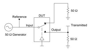
Channel switch control/s test socket is normalized. Off isolation is measured across an off channel. On loss is the bandwidth of an On switch.  $V_{\text{ISO}}$ , Bandwidth and  $V_{\text{ONL}}$  are independent of the input signal direction.
