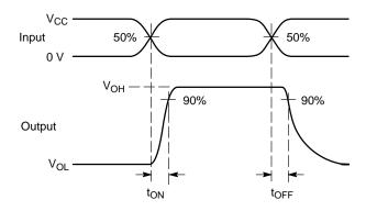
Figure 3. t<sub>ON</sub>/t<sub>OFF</sub>
