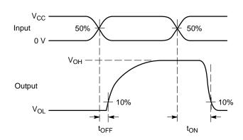
Figure 4. t<sub>ON</sub>/t<sub>OFF</sub>
