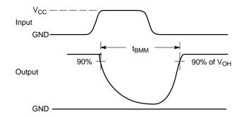
Figure 2. t<sub>BBM</sub> (Time Break-Before-Make)
