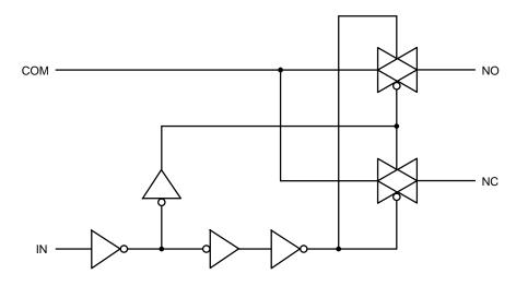
Figure 1. Logic Equivalent Circuit
