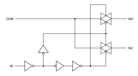
Figure 1. Logic Equivalent Circuit
