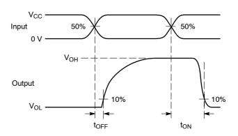
Figure 4. t<sub>ON</sub>/t<sub>OFF</sub>
