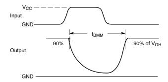
Figure 2. t<sub>BBM</sub> (Time Break–Before–Make)
