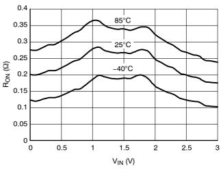
Figure 10. On–Resistance vs. Input Voltage @ V<sub>CC</sub> = 3.0 V
