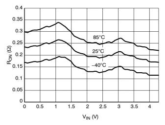
Figure 11. On–Resistance vs. Input Voltage @ V<sub>CC</sub> = 4.3 V
