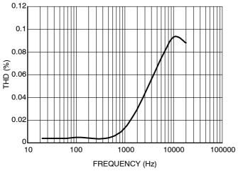
Figure 9. Total Harmonic Distortion
