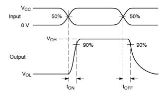
Figure 3. t<sub>ON</sub>/t<sub>OFF</sub>
