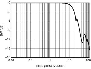
Figure 8. Bandwidth vs. Frequency
