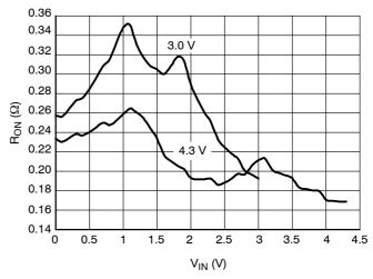
Figure 12. On-Resistance vs. Input Voltage
