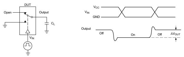
Figure 6. Charge Injection: (Q)
