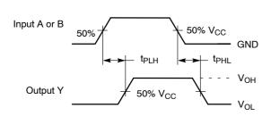
Figure 3. Switching Waveforms
