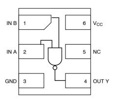
Figure 1. Pinout (Top View)
