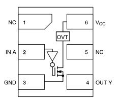
Figure 1. Pinout (Top View)
