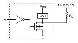
Figure 5. Output Voltage Mismatch Application
