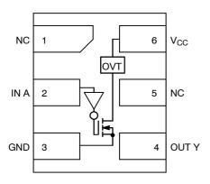
Figure 1. Pinout (Top View)
