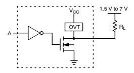
Figure 5. Output Voltage Mismatch Application
