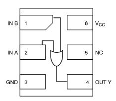
Figure 1. Pinout (Top View)
