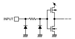
Figure 7. Input Equivalent Circuit
