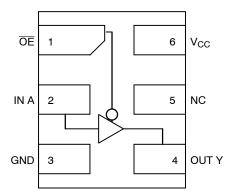
Figure 1. Pinout (Top View)
