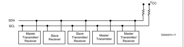
Note: Due to open drain configuration of SDA, a bus-level resistor is called for (Typical value =  $4.7\Omega$ )
