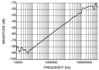
Figure 5. Off–Channel Isolation @  $V_{CC}$  = 5.5 V,  $25^{\circ}C$
