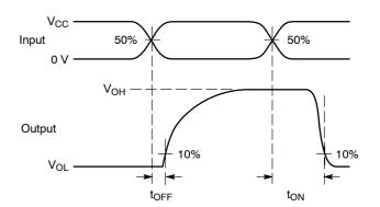
Figure 2.  $t_{ON}/t_{OFF}$
