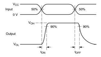
Figure 1. t<sub>ON</sub>/t<sub>OFF</sub>
