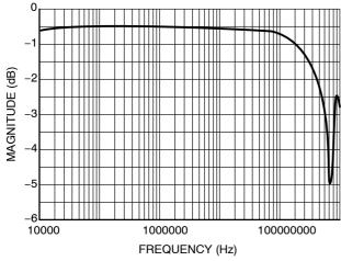
Figure 4. Typical Bandwidth @  $V_{CC} = 5.5 V$ ,  $25^{\circ}C$
