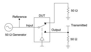
Channel switch control/s test socket is normalized. Off isolation is measured across an off channel. On loss is the bandwidth of an On switch.  $V_{ISO}$ , Bandwidth and  $V_{ONL}$  are independent of the input signal direction.
