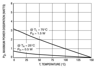
Figure 5. Steady State Power Derating
