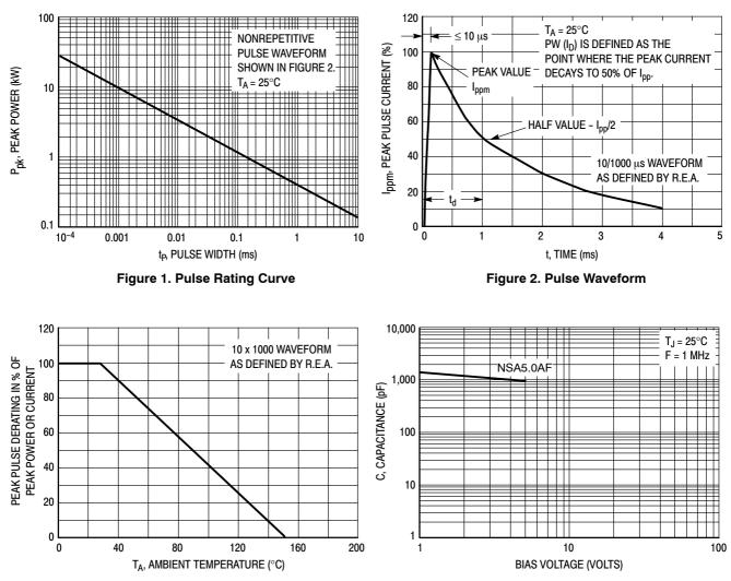
Figure 3. Pulse Derating Curve
