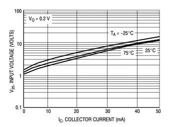
Figure 11. Input Voltage versus Output Current
