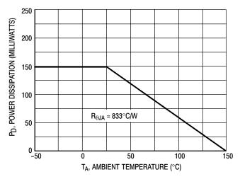
Figure 1. Derating Curve
