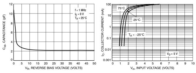
Figure 4. Output Capacitance
