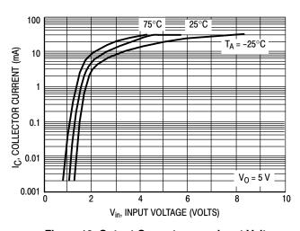
Figure 10. Output Current versus Input Voltage
