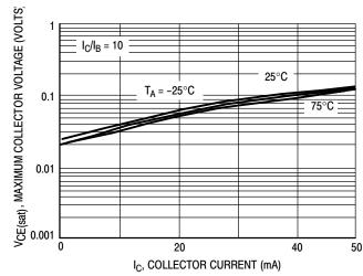
Figure 7. V<sub>CE(sat)</sub> versus I<sub>C</sub>
