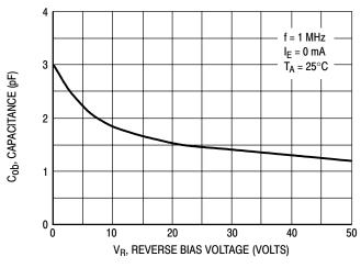
Figure 9. Output Capacitance
