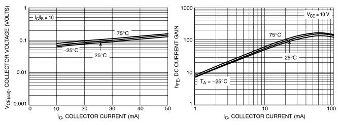
Figure 2.  $V_{CE(sat)}$  versus  $I_C$
