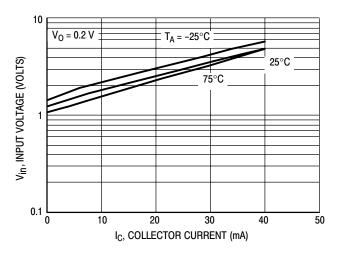
Figure 6. Input Voltage versus Output Current
