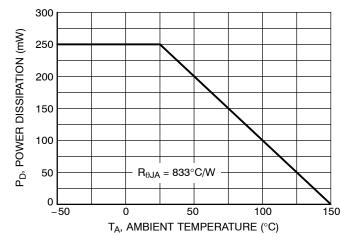
Figure 1. Derating Curve
