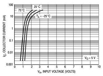
Figure 5. Output Current versus Input Voltage
