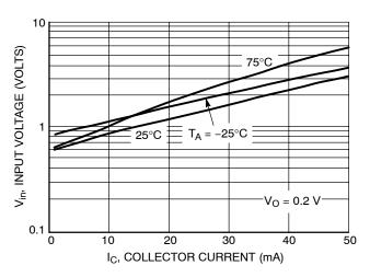
Figure 11. Input Voltage versus Output Current
