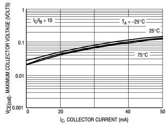
Figure 2. V<sub>CE(sat)</sub> versus I<sub>C</sub>
