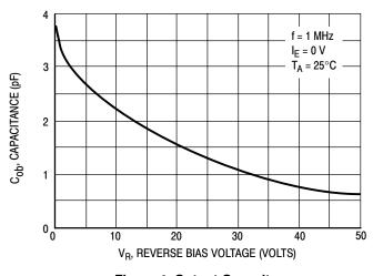
Figure 4. Output Capacitance
