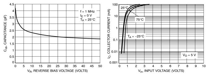
Figure 9. Output Capacitance
