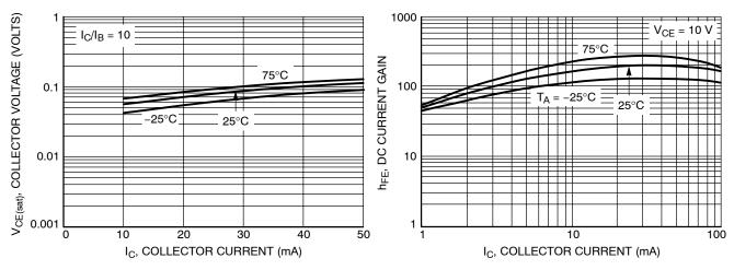
Figure 7.  $V_{CE(sat)}$  versus  $I_C$
