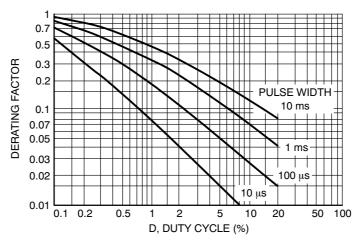
Figure 5. Typical Derating Factor for Duty Cycle
