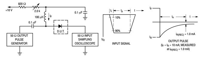
Notes: 1. A 2.0 k $\Omega$  variable resistor adjusted for a Forward Current (I<sub>F</sub>) of 10 mA. 2. Input pulse is adjusted so I<sub>R(peak)</sub> is equal to 10 mA.
