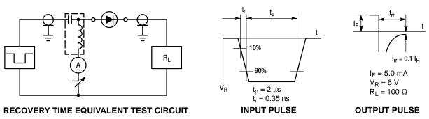
Figure 4. Reverse Recovery Time Test Circuit for the NSDEMP11XV6T1
