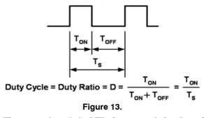
The current through the LEDs is constant during the period they are turned on resulting in the light being consistent with no shift in chromaticity (color). The brightness is in proportion to the percentage of time that the LEDs are turned on.
