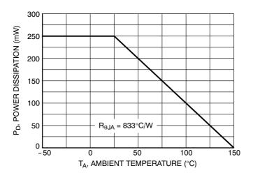
Figure 1. Derating Curve
