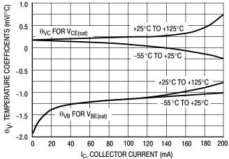
**Figure 15. Temperature Coefficients**
