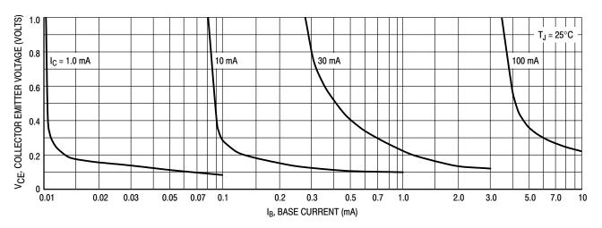
Figure 13. Collector Saturation Region
