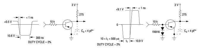
\* Total shunt capacitance of test jig and connectors
