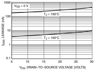
Figure 6. Drain-to-Source Leakage Current vs. Voltage
