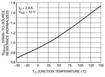
Figure 5. On–Resistance Variation with Temperature
