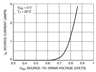
Figure 10. Diode Forward Voltage vs. Current
