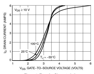
Figure 2. Transfer Characteristics
