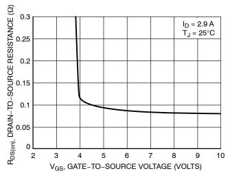
Figure 3. On-Resistance vs. Gate-to-Source Voltage
