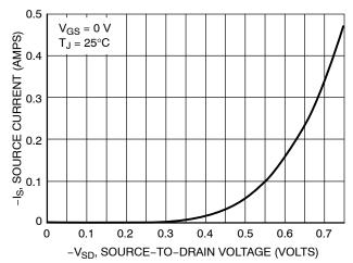
Figure 10. Diode Forward Voltage vs. Current
