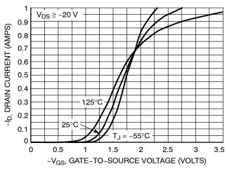
Figure 2. Transfer Characteristics
