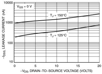
Figure 6. Drain-to-Source Leakage Current vs. Voltage
