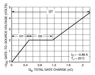
Figure 8. Gate-to-Source Voltage vs. Total Gate Charge
