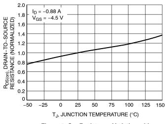
Figure 5. On–Resistance Variation with Temperature
