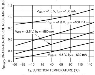
Figure 5. On–Resistance Variation with Temperature
