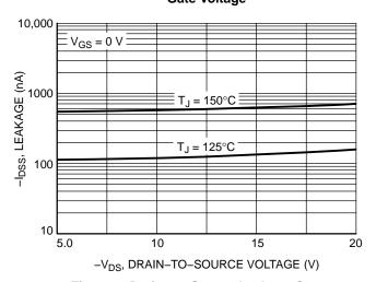
Figure 6. Drain-to-Source Leakage Current vs. Voltage
