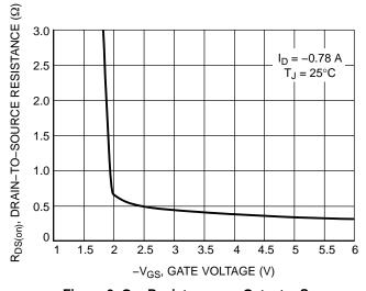
Figure 3. On-Resistance vs. Gate-to-Source Voltage
