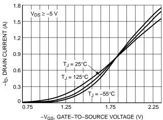
Figure 2. Transfer Characteristics
