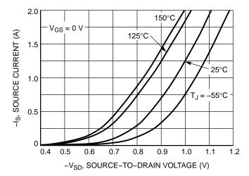
Figure 9. Diode Forward Voltage vs. Current
