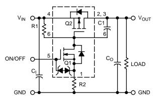
Figure 12. Load Switch Application
