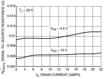
Figure 3. On-Resistance vs. Gate-to-Source Voltage
