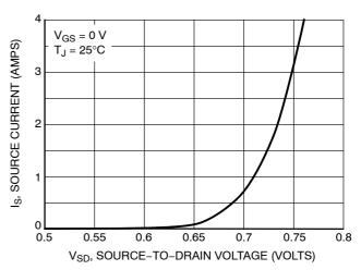
Figure 10. Diode Forward Voltage vs. Current
