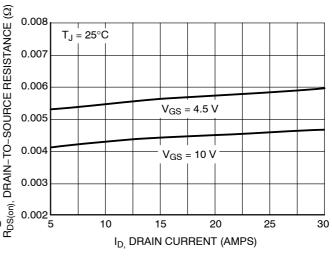
Figure 3. On-Resistance vs. Gate-to-Source Voltage
