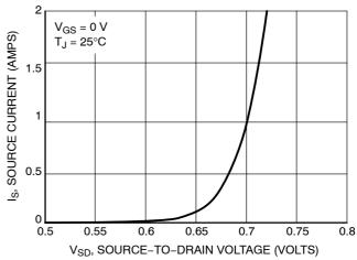
Figure 10. Diode Forward Voltage vs. Current
