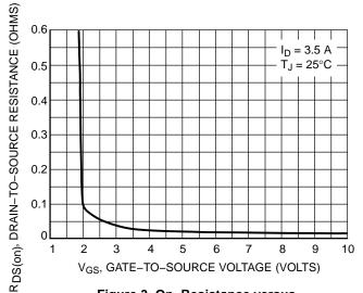
Figure 3. On–Resistance versus Gate–To–Source Voltage
