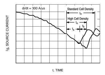
Figure 11. Reverse Recovery Time (t<sub>rr</sub>)
