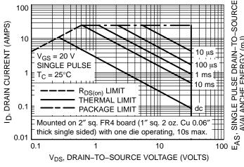
Figure 12. Maximum Rated Forward Biased Safe Operating Area
