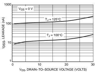
Figure 6. Drain-To-Source Leakage Current versus Voltage
