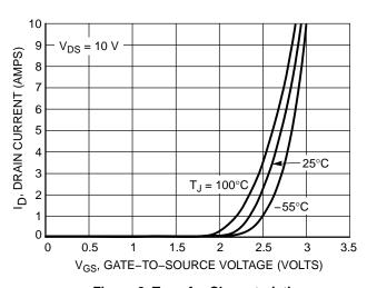
Figure 2. Transfer Characteristics
