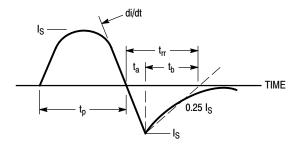
Figure 15. Diode Reverse Recovery Waveform
