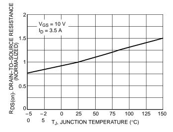
Figure 5. On–Resistance Variation with Temperature
