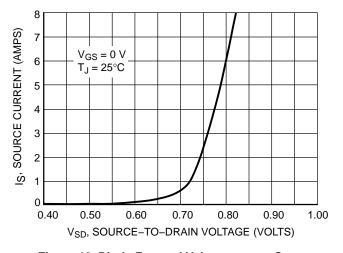
Figure 10. Diode Forward Voltage versus Current
