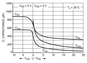
GATE-TO-SOURCE OR DRAIN-TO-SOURCE VOLTAGE (VOLTS)
