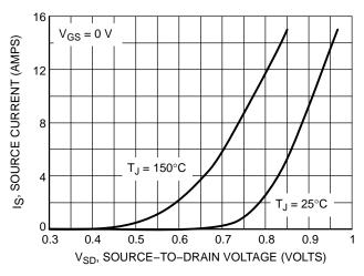
Figure 10. Diode Forward Voltage versus Current
