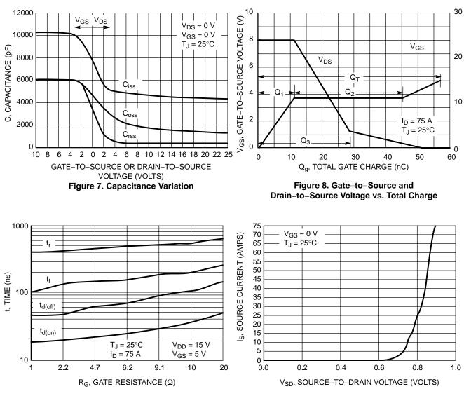
Figure 9. Resistive Switching Time Variation vs. Gate Resistance
