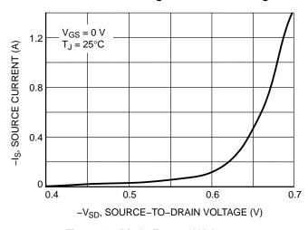
Figure 10. Diode Forward Voltage versus Current
