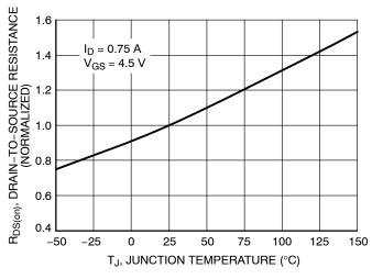
Figure 5. On–Resistance Variation with Temperature
