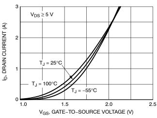
Figure 2. Transfer Characteristics
