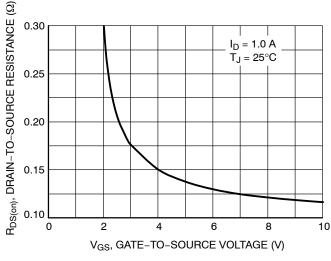
Figure 3. On-Resistance vs. Gate-to-Source Voltage
