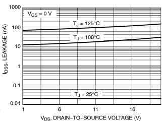
Figure 6. Drain-to-Source Leakage Current vs. Voltage
