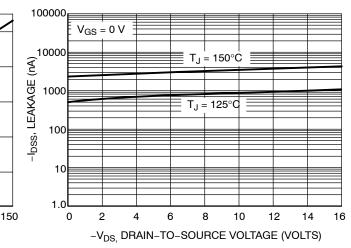
Figure 6. Drain-to-Source Leakage Current vs. Voltage
