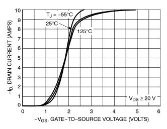
Figure 2. Transfer Characteristics
