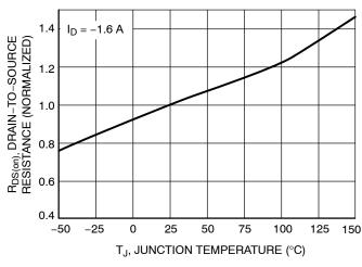
Figure 5. On–Resistance Variation with Temperature
