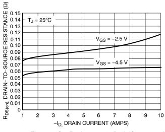
Figure 4. On–Resistance vs. Drain Current and Temperature
