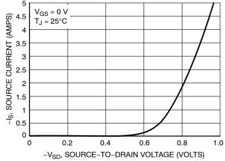
Figure 10. Diode Forward Voltage vs. Current
