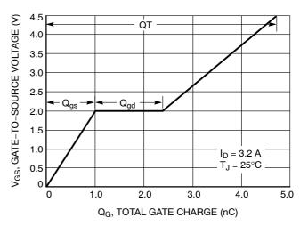
Figure 8. Gate-to-Source Voltage vs. Total Charge
