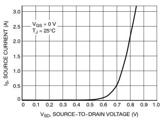
Figure 10. Diode Forward Voltage vs. Current
