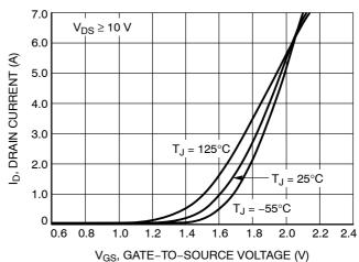
Figure 2. Transfer Characteristics
