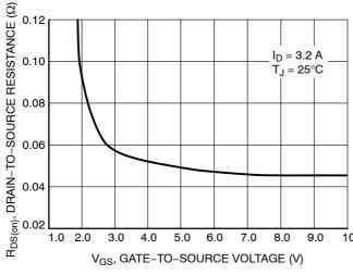
Figure 3. On-Resistance vs. Gate Voltage
