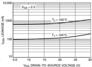
Figure 6. Drain-to-Source Leakage Current vs. Voltage
