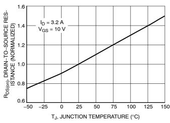
Figure 5. On–Resistance Variation with Temperature
