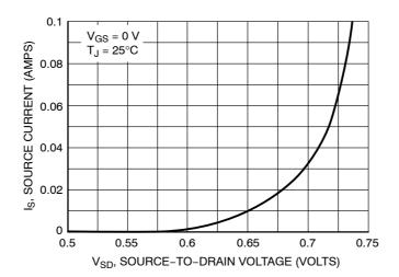
Figure 9. Diode Forward Voltage vs. Current
