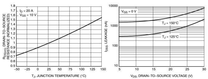
Figure 5. On–Resistance Variation with Temperature
