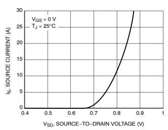
Figure 10. Diode Forward Voltage vs. Current
