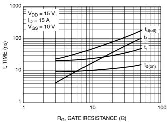
Figure 9. Resistive Switching Time Variation
