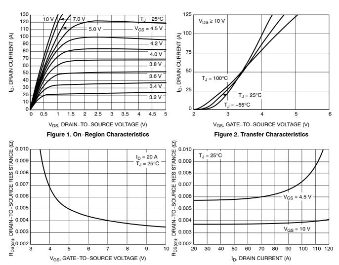
Figure 3. On-Resistance vs. Gate-to-Source Voltage
