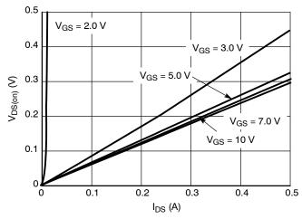
Figure 2.  $\rm V_{DS(on)}$  Variation with  $\rm I_{DS}$  and Gate Voltage
